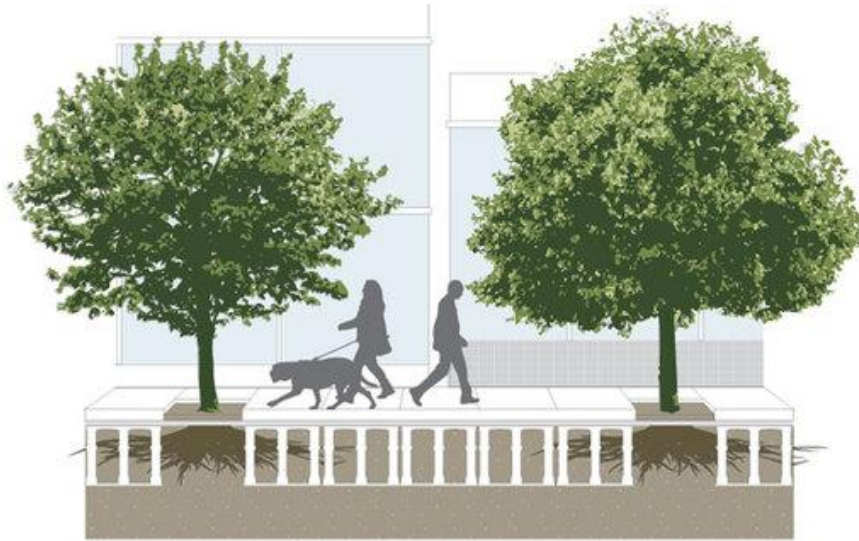
Image: Suspended pavement system.
